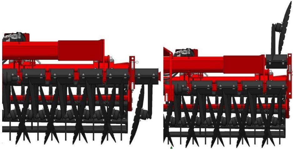
**Figure 3.** Working and transport positions (folded side sections)
